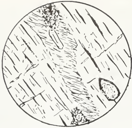
Figure 8. Amphibole schist from north of Deadwood Creek as seen in thin-section. Development of chlorite along cleavage in hornblende; minor aggregates and euhedra of sphene. X 175.
